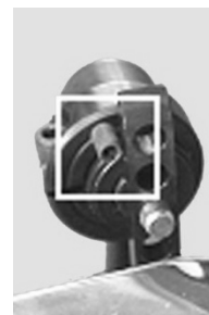
Right side (close up, inside): Down Stop rests against the top/front of the L-bar to limit the “down” motion
