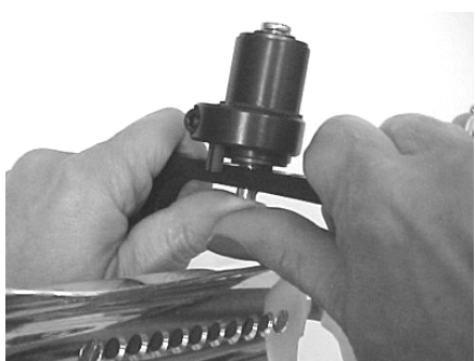
Pressing out pivot pin with thumbs.
