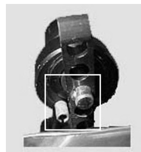
Left side (close up, inside): Down Stop rests against the bottom/rear of the L-bar to limit the “down” motion
