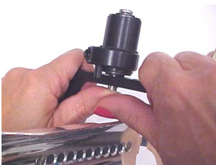
Pressing out pivot pin with thumbs.
