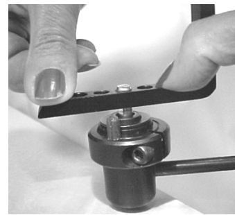
Reattaching L-bar with Down Stop in front.
