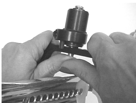
Pressing out pivot pin with thumbs.
