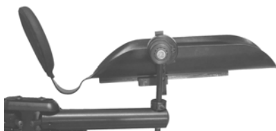
Slide positioned so forearm support is balanced.
