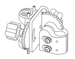
When optimal functional use of the mobile arm support is achieved, tighten the **Locking Set Screws** using the small T-Wrench. This will lock the mount in its position on the wheelchair upright (back post).
