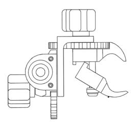
1. Loosen clamp screws with large T-Wrench (Do not remove screws!) and open clamps to their widest position by pushing the moveable jaw forward and pulling it outward as shown in picture.
