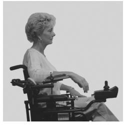
Loosen lock knob "B" and rotate scroll wheel "B" to adjust posterior tilt (reaching backward).
