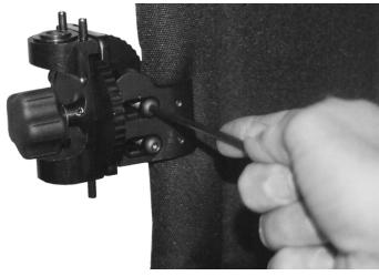
3. Tighten clamp screws with Scroll Wheel "B" in line with the arm rest of the wheelchair.
