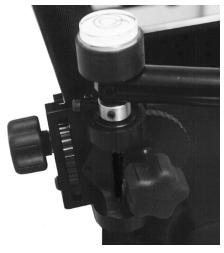
4. Insert **Bubble Level** (sold separately) through the ball bearings of the mount. Adjust the mount so that the bubble level is neutrally balanced (bubble is in or close to center ring of level).
